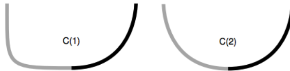
Figure 11: C(1) and C(2) continuity across two curve segments 9
