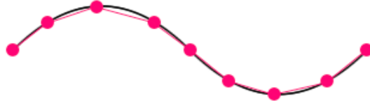
Figure 12: The path that approximate curve length is calculated from.
